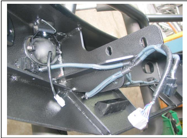
Figure 9: Parking sensor mounted into protection bar. NOTE wiring direction secured to mount.
