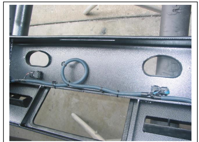
Figure 8: Parking sensor mounted into protection bar with secured wiring.
